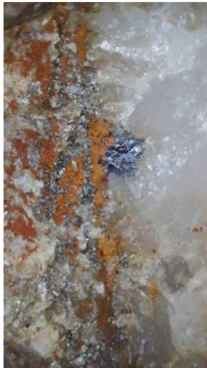
Figure 3 showing on the left a grain of gold and on the right side a grain of galena, (grains are approximately 1mm in diameter).
