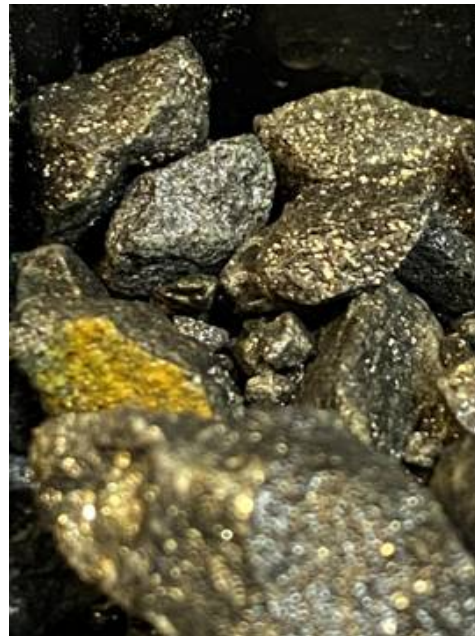
Figure 4: Photograph of coarse chalcopyrite + pyrite in RC chips MHRC0029 64-66m grading 1.7% Cu.
